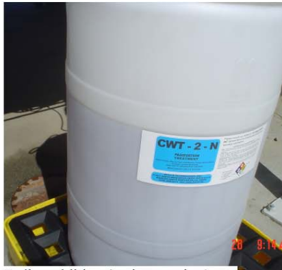
Boiler additive (anti-corrosion)
