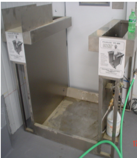
Foot Sanitizer Mixing Unit
